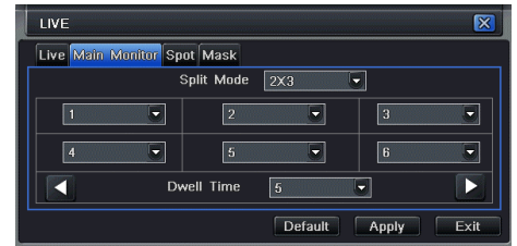
Fig 4-8 Live Configuration-Main Monitor
